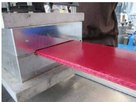
Figure 3: Fiber-reinforced composite exiting from the heated pultrusion die
