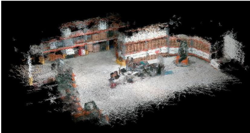
**Scope:** The [ARIBIC Project](#) is a German-Canadian cooperation project to research the application of AI Methods in warehouses. The goal is to obtain information about the condition of a logistics center with the help of the navigation sensors on automated guided vehicles. In the end, a living digital twin of the logistics center should be created.
